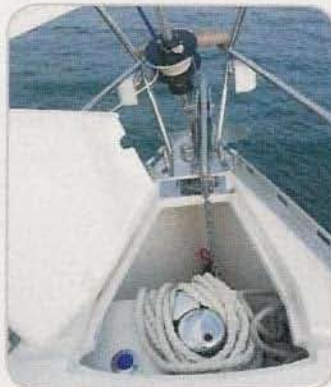
Clockwise from above: Deep chain locker with windlass; big wheel with cutaway seating; her stern platform is large and easily accessed; her high boom carries a fully battened mainsail in a lazybag; she has both shallow and full depth cockpit lockers for all the usual cruising clobber.
